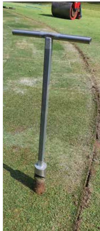
The site green assessment revealed that the green has 100mm of sand without any proper drainage, which we will improve to meet USGA specifications.
